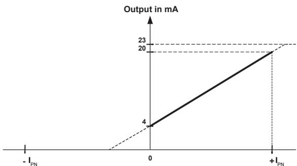
**Note:** <sup>1)</sup> The performance specified in the datasheet is valid within the 4-20 mA output range only.
